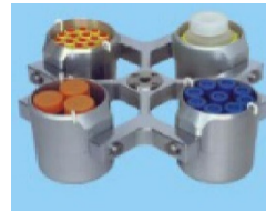
Kapasite: 4x500ml Maks. Hız: 4000rpm Maks. RCF: 3040xg
